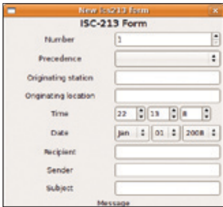
Figure 4 — An ISC-213 form ready to be filled out for transmission over D-RATS .
