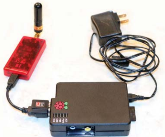
A Raspberry Pi 1B Connected to an Internet Labs DV Access Point Dongle (left) to Form a D-STAR Access Point. Also Seen Here Are the Micro WIFI USB Adapter (in the left side of the RPi), SDHC Card (in the right side) and the USB Power Supply.
