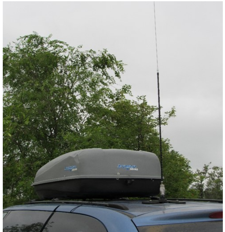
Figure 1 – The 20m hamstick on top of the van. Visible at the base of the antenna is a mobile whip spring (used for flexibility for the antenna) and the MFJ triple magnet mount.
