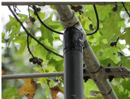
A close up of the author's 2-meter yagi secured to the top of the mast.
