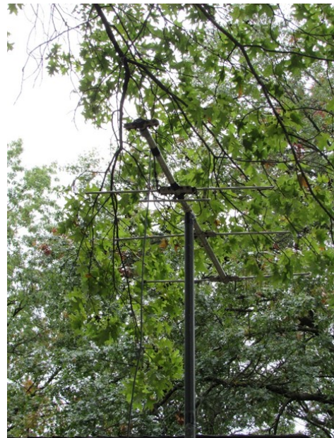
The modified 2-meter yagi, now with 3 elements instead of 4 elements.
