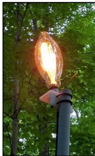
Due to a difference in SWRs the power in each bulb of an array was not the same.
