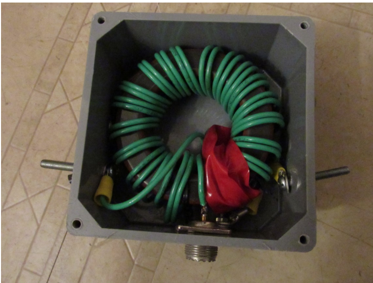
Figure 4: Interior of homebrew insulation transformer
