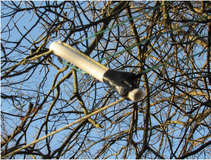
Figure 3: PVC spreader and support rope
