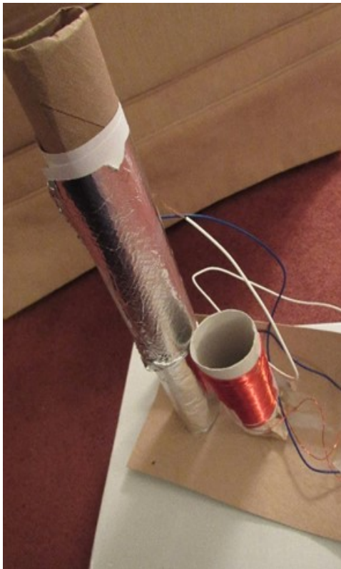
Figure 1 — One of the author's homemade crystal radios, built from a kit.
