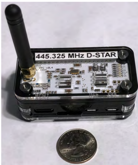
ZUMspot Running the Pi-Star software (US Quarter for Size Comparison)
